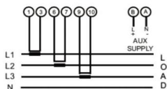
Connect external current transformer secondary of Nano CT to meter as shown below.
