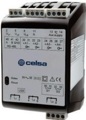
DIN rail, fully programmable, high accuracy, the multi-transducer, can be used with 50, 60 or 16 $\frac{2}{3}$  Hz rated frequencies with a wide range of AC and DC auxiliary supply. This transducer can measure active and reactive powers, power factors, and all other electrical quantities including voltage and current for any 3-phase system. The CPQT can be easily programmed through its USB micro standard port and ConfigLQT free software.
